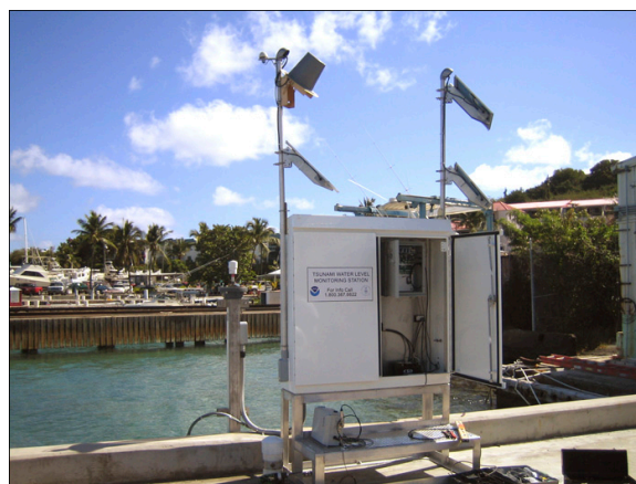
Figure 17. Tsunami tide station in Christiansted, Virgin Islands.
