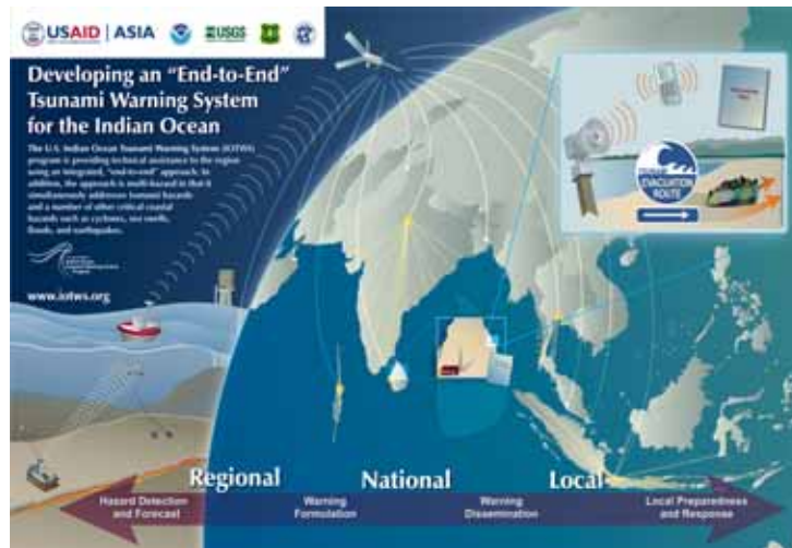
Figure 2.1 Components of a Tsunami Early Warning System
