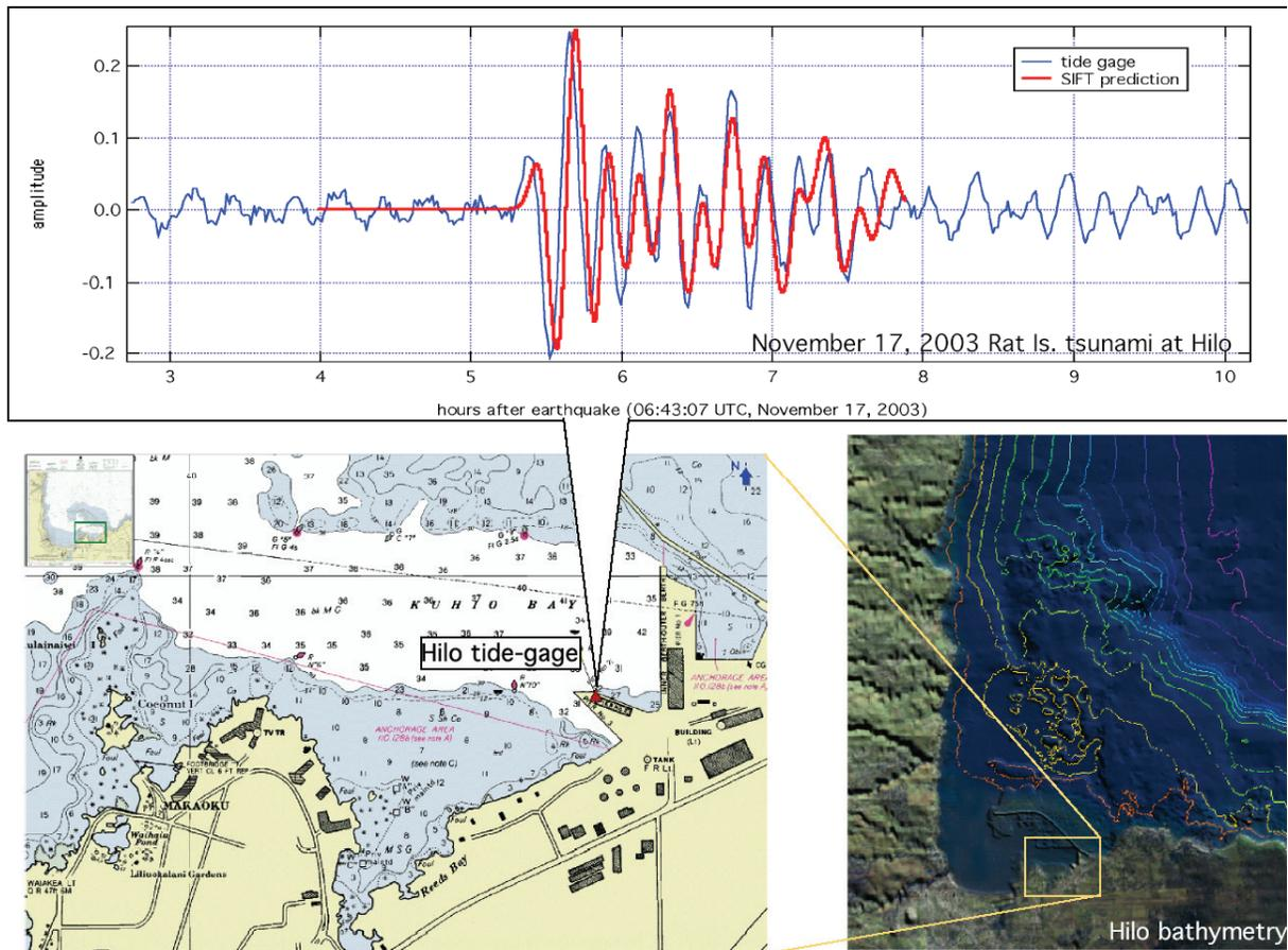
**Figure 7. Coastal forecast at Hilo, HI for 2003 Rat Island tsunami. Top frame shows comparison of the forecasted (red line) and measured (blue line) gage data. Bottom frames shows location of Hilo tide-gage and digital elevation data for the high-resolution inundation computation.**
