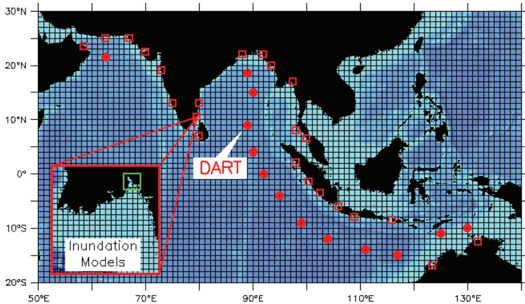
**Figure 13. Elements for tsunami forecasts, including tsunameter data ingested into a set of numerical models that telescope to a local community.**
