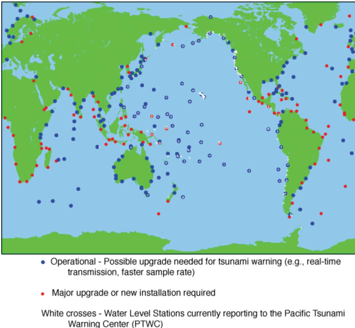
**Figure 4. Location of tide gauges that are in use or can be modified for tsunami warning.**
