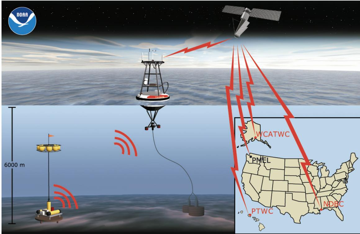
**Figure 5. Deep Ocean Assessment and Reporting of Tsunami (DART) tsunameter technology.**
