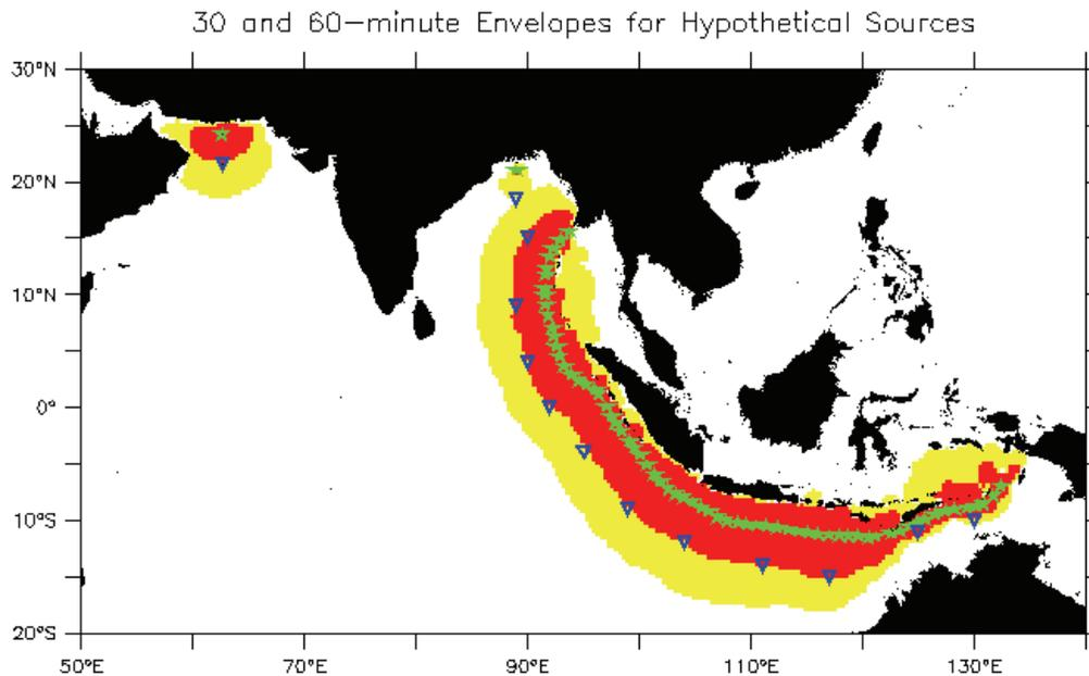
**Figure 12 Potential tsunami sources (green stars) are used to produce 30 minute (red area) and 1 hour (yellow area) travel times. A network of DART buoys (blue triangles) can detect tsunamis from these sources within 1 hour.**
