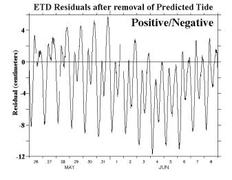
The mean of the absolute value of the residuals for the data from the ETD for the dates of May 26- June 9 is 3.52 centimeters, which falls with the <5cm design capability. The plot of the values from which this was calculated is shown below.
