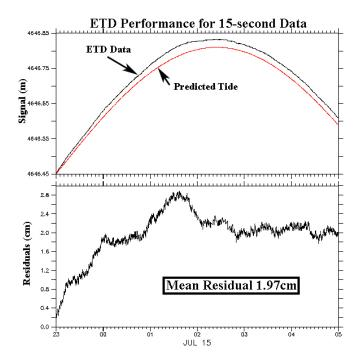
11. Other Bottom Pressure Recorder (BPR) commands tests: At least one successful test for each of the following during 120 day evaluation period.
