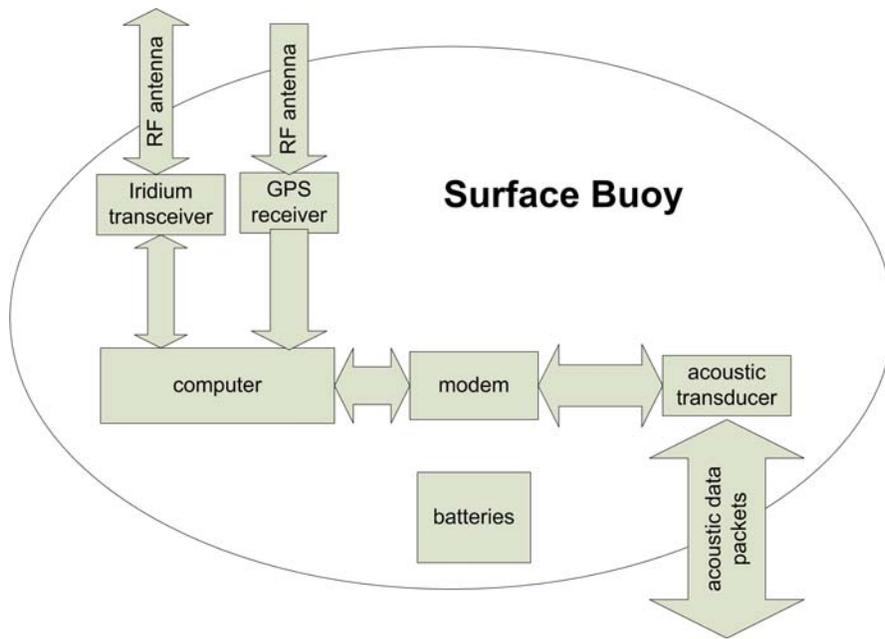
**Figure 5: Block diagram of DART II surface buoy.**
