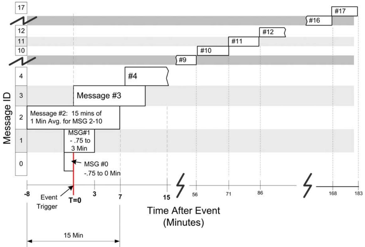
**Figure 6: Timing diagram showing messages during Event Mode.**
