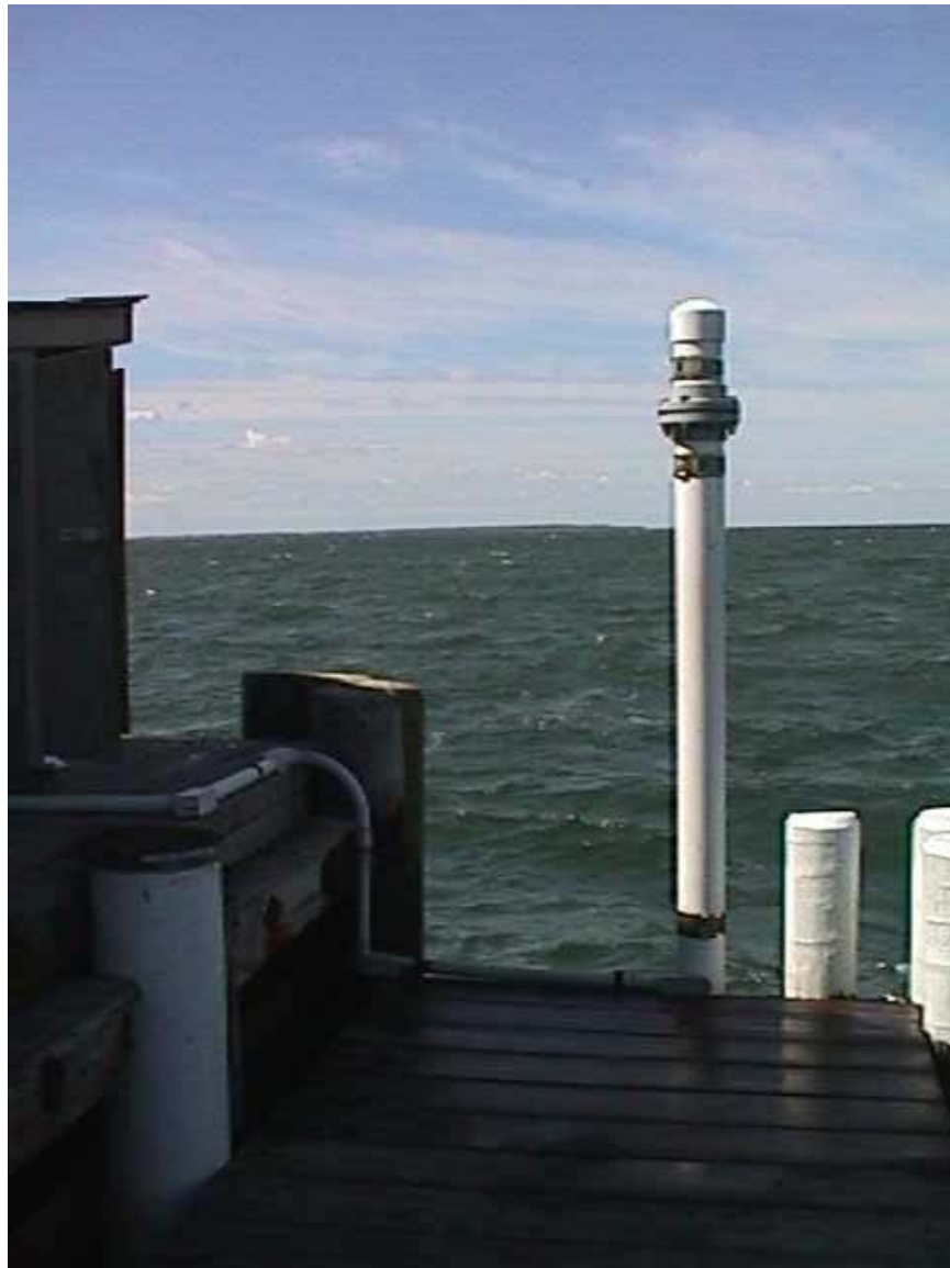
Figure 5. Photo of tide gauge located at the NE corner of the Rough Rider Condominium Pier.
